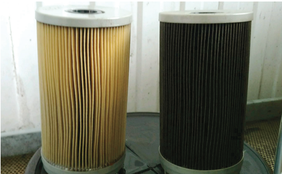
Two fuel filters from Red Mountain Trucking's fleet. The filter on the left has 20,000 miles on it while the filter on the right has 10,000 miles. The dirty filter is from a truck not treated with CarbonTreat™.
